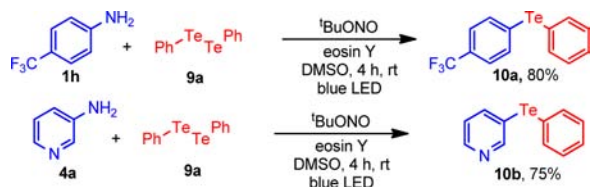
Scheme 9. Visible Light Photocatalyzed Synthesis of Tellurides
